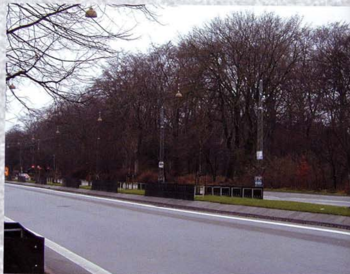
Figure 8. Landscapers and urban foresters in Denmark use these barriers to prevent road salt build-up in soils along roadways near Copenhagen. Photo courtesy of Lars Bo Pedersen.
