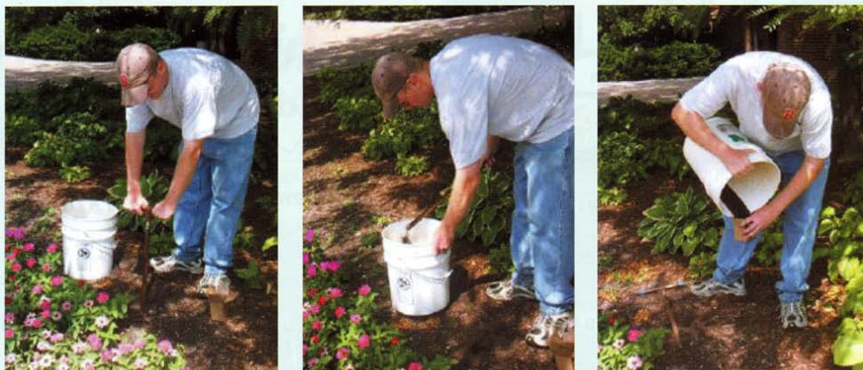
Figure 3. Soil samples can be collected with a soil probe (shown), a trowel or a shovel. Take 10-15 samples, mix them together in a clean bucket and pour sample into a soil test box or a ziplock baggie.
